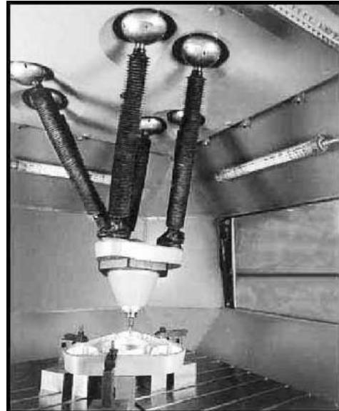
6.13-rasm. Stend-simulyator platformasi dizayni uchun pastki ko‘rinish.
