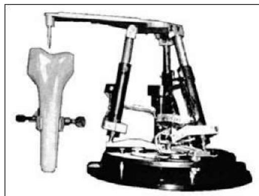
6.16-rasm. Suyakning sirtini tekshiruvchi tripod
