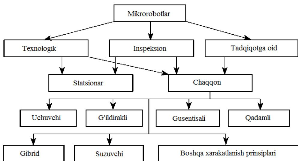
6.3-rasm. Mikrotobotlarning tasnifi
