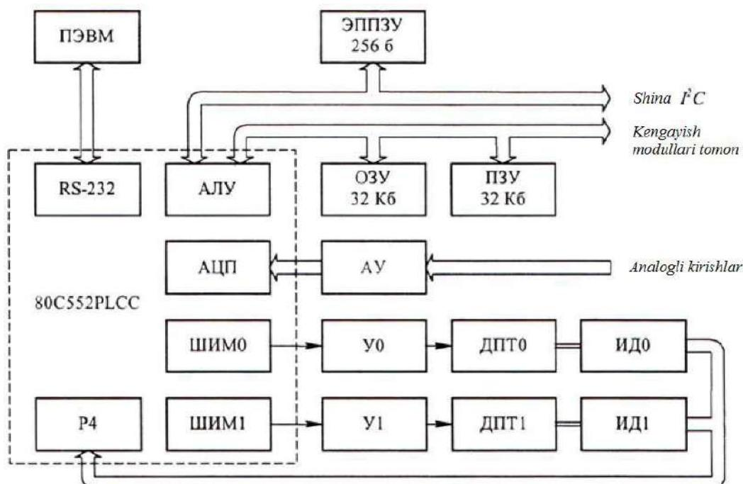
5.14-rasm. MPSU TR ning funksional sxemasi
